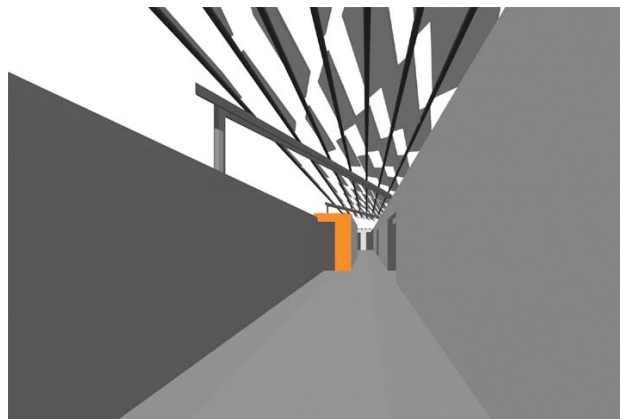
Figure 9: On March 21st and September 21st the sun leaves a mark on a west facing wall as it sets due west.
